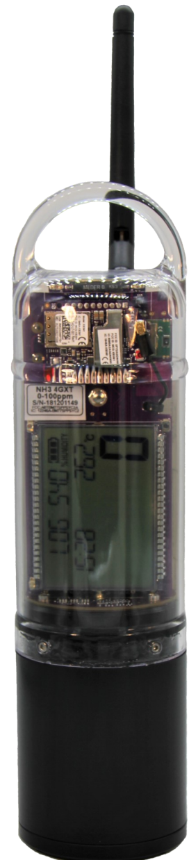
Acrulog NH3 PPM logger with 4G and external antenna
